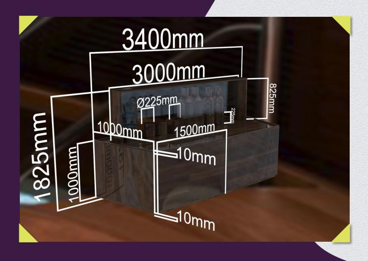
My idea was a pop-up minibar, that would rise from the refrigerated table. This would keep the glasses and bottles safely stowed, and chilled while sailing, then popping out into a functioning minibar when stationary.
